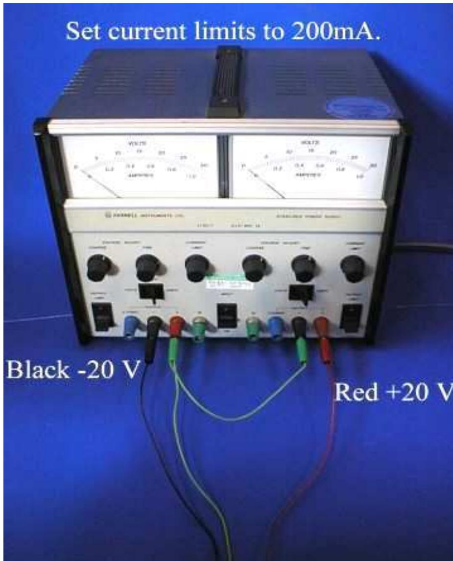
**Photo 5.2.** Power supply connections
