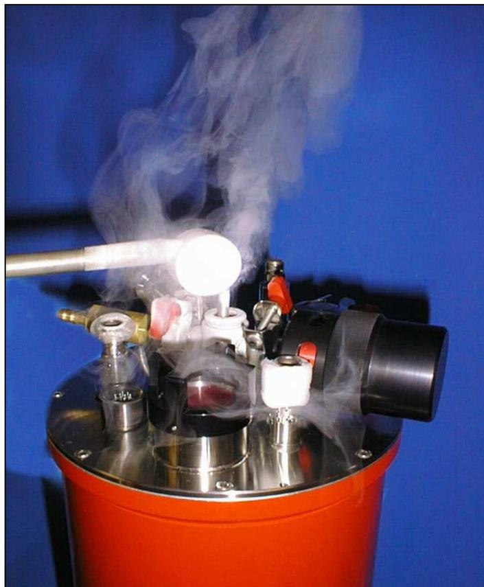
**Photo 4.2.** Helium gas exhaust during fill
