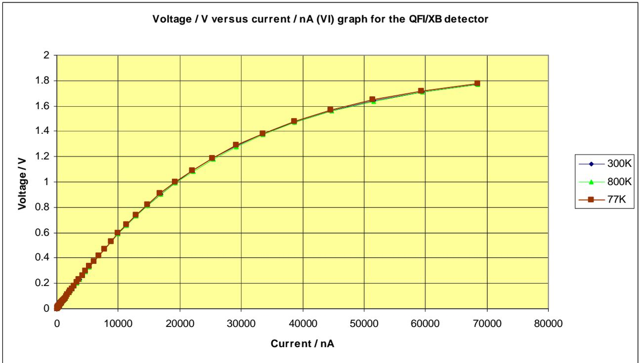
**Fig. 6.4.** The detector system VI characteristic measured with both a 77K, 300K and a 800K dc load
