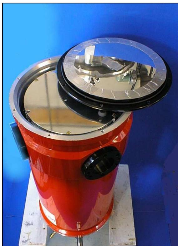
**Photo 1.4.** Liquid nitrogen base-plate in position
