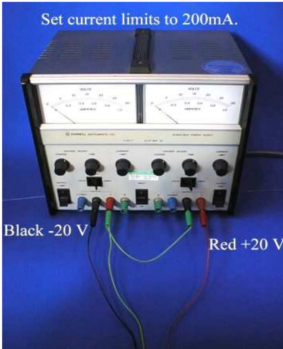
**Photo 5.2.** Power supply connections
