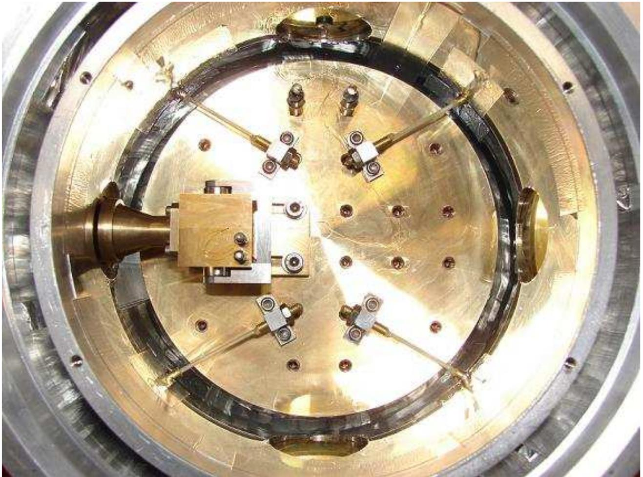
**Photo 1.2b.** The inside view of the tuned InSb detector system
