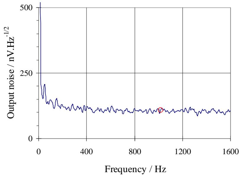
**Fig. 5.1a.** Typical preamplifier input shorted noise spectra
