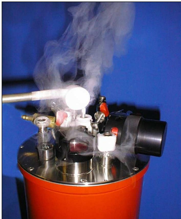
**Photo 4.2.** Helium gas exhaust during fill
