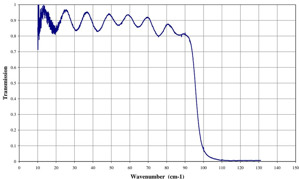
**Fig. C1.** Transmission spectrum for the type QMMF 100cm<sup>-1</sup> low pass filter
