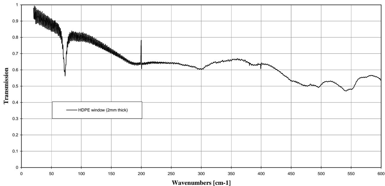
**Fig. C.2.** Measured transmission of a 2mm thick HDPE window from 20cm<sup>-1</sup> to 600cm<sup>-1</sup>. The polyethylene characteristic absorption increase is clearly seen around 73cm<sup>-1</sup>.
