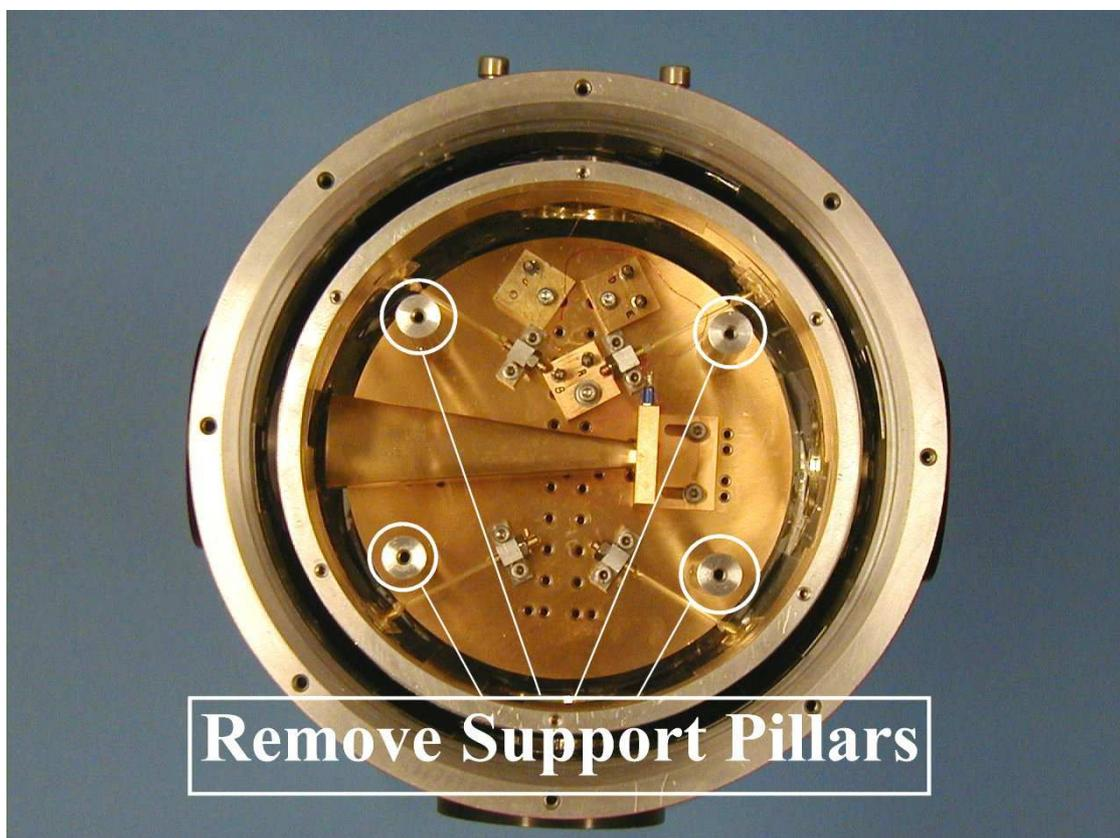
**Photo 1.2a.** The four support pillars and the detector optics
