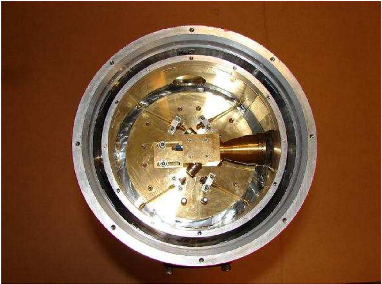
**Photo 1.2b.** The inside view of a tuned InSb detector system
