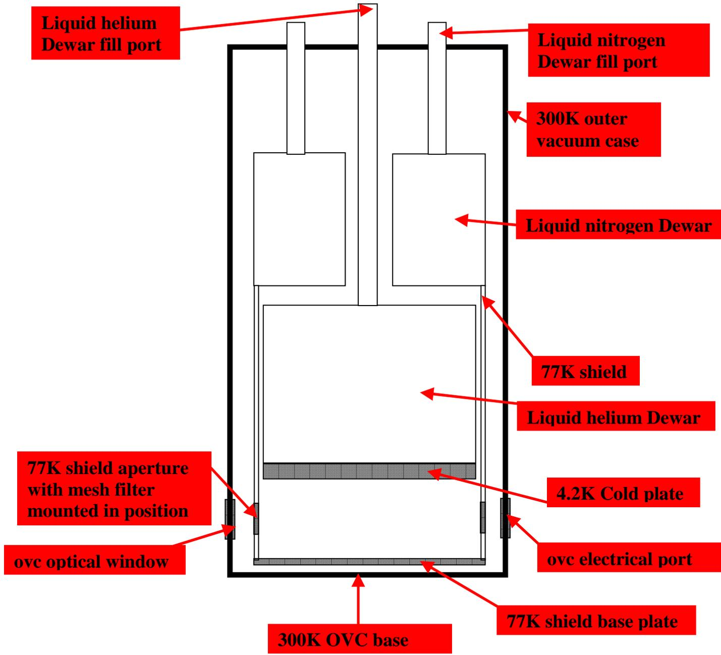
**Fig. 1.1.** Schematic showing the main features of the cryostat. Not to scale
