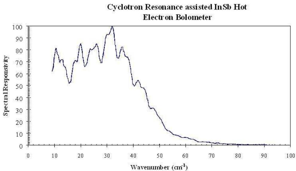
**Fig. A.2.** Spectral responsivity of the Type QFI/XBI detector
