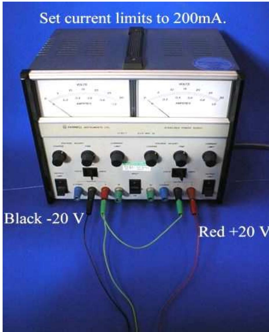
**Photo 5.2.** Power supply connections
