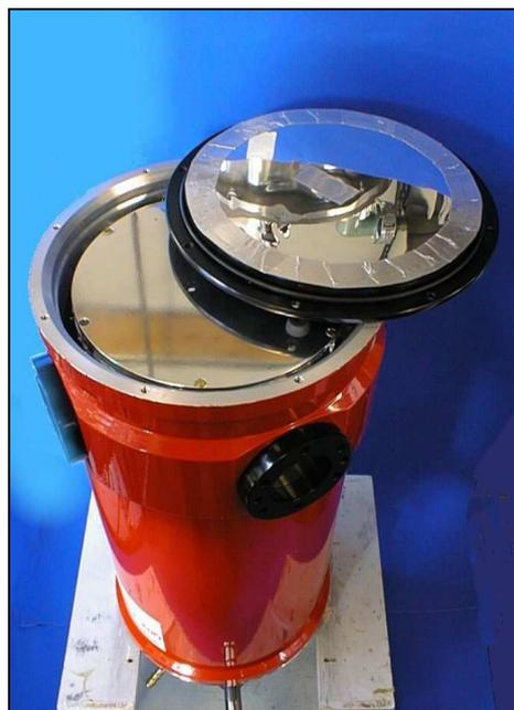
**Photo 1.4.** Liquid nitrogen base-plate in position
