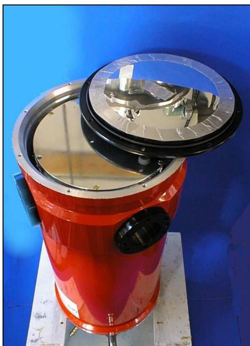
**Photo 1.4.** Liquid nitrogen base-plate in position
