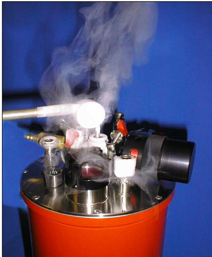
**Photo 4.2.** Helium gas exhaust during fill
