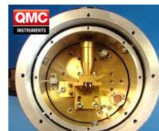
Cryostat and bolometer
