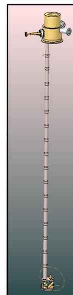
TK has manufactured two 94 GHz probes for ESR and DNP-NMR, using two refocussing mirrors to feed the beam to the sample holder from below, allowing a sample changer mechanism to extract the sample from above.
