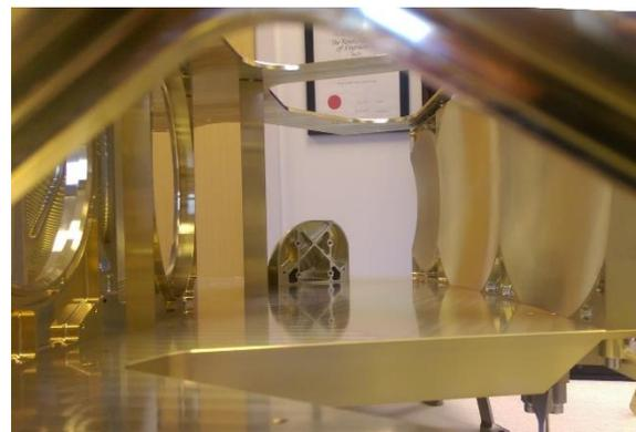
Inside the Quasi Optic Network (QON) Engineering Qualification Model for the MetOp-SG satellite MWS instrument
