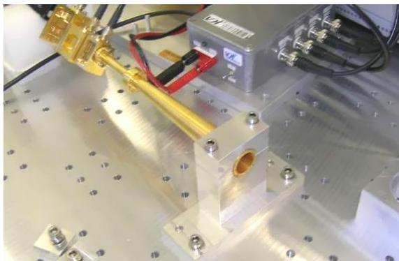
TK Ultra-Gaussian gold-plated copper feed horn with VDI waveguide-based multipliers
