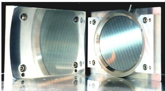
A curved refocusing mirror (left) and a rotatable wire-grid polarizer (right)
