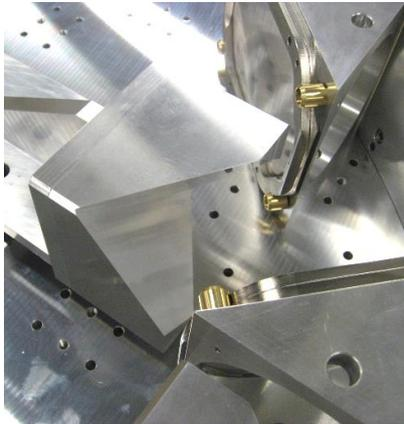
Diagonal roof mirror – part of a Martin-Puplett interferometer for NIH (USA)
