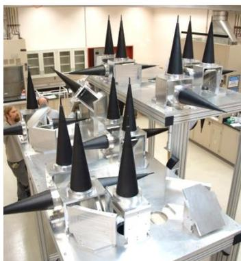
TK collaborated with the Millimetre Wave & EPR group on the HiPER project, a 94 GHz kilowatt pulsed ESR spectrometer. It has the ability to perform ESR and certain DNP-NMR experiments. The quasi optics in this spectrometer help to give it a very short dead time by reducing standing waves. HiPER spectrometers have now also been supplied to PNNL (USA) and FSU for NHMFL (USA).
