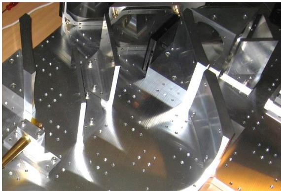
Refocusing and flat mirrors on a standard TK 125 mm grid bench plate
