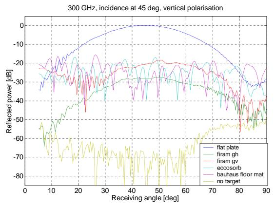
Figure 5.5 Scattered power as a function of the receiving angle (vertical polarisation at 300 GHz,  $\theta_i = 45^{\circ}$ ).
