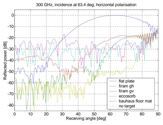
Figure 5.8 Scattered power as a function of the receiving angle (horizontal polarisation at 300 GHz,  $\theta_i = 63.4^{\circ}$ ).
