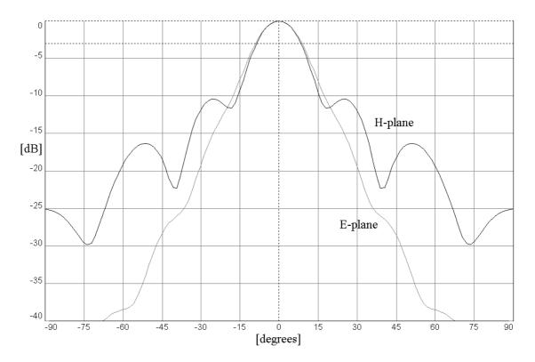
Figure 4.18 Theoretical E- and H-plane directional patterns of the 200 GHz horns.
