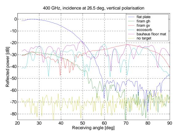
Figure 5.9 Scattered power as a function of the receiving angle (vertical polarisation at 400 GHz,  $\theta_i = 26.5^{\circ}$ ).
