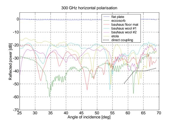
Figure 4.11 Reflectivity as a function of the specular angle at 300 GHz and horizontal polarisation.
