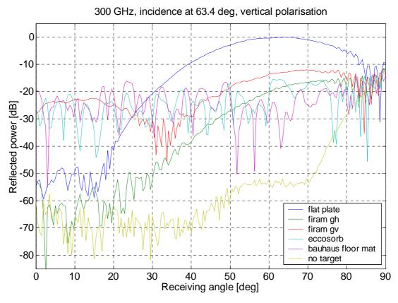
Figure 5.7 Scattered power as a function of the receiving angle (vertical polarisation at 300 GHz,  $\theta_i = 63.4^{\circ}$ ).
