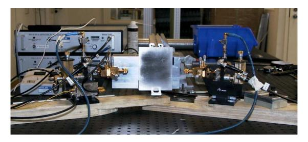
Figure 4.7 Photograph of the test bench with surrounding absorbers removed (calibration target at 600 GHz, vertical polarisation).
