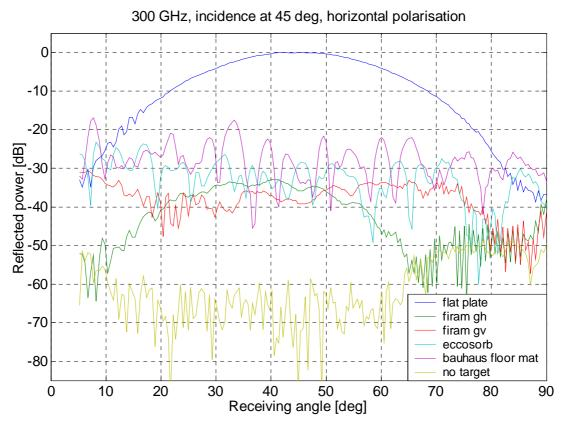
Figure 5.6 Scattered power as a function of the receiving angle (horizontal polarisation at 300 GHz,  $\theta_i = 45^{\circ}$ ).
