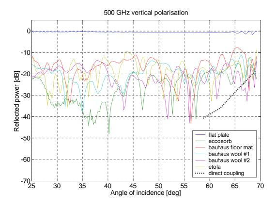
Figure 4.14 Reflectivity as a function of the specular angle at 500 GHz and vertical polarisation.
