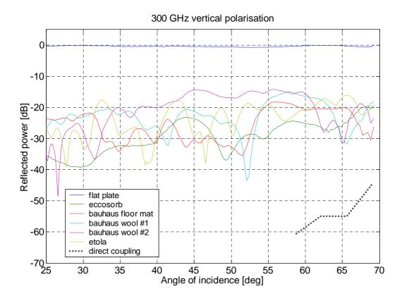
Figure 4.10 Reflectivity as a function of the specular angle at 300 GHz and vertical polarisation.
