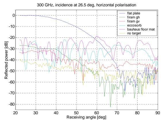
Figure 5.4 Scattered power as a function of the receiving angle (horizontal polarisation at 300 GHz,  $\theta_i = 26.5^{\circ}$ ).
