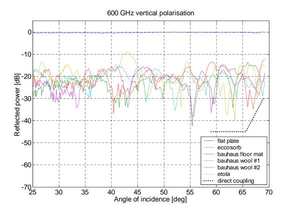
Figure 4.16 Reflectivity as a function of the specular angle at 600 GHz and vertical polarisation.
