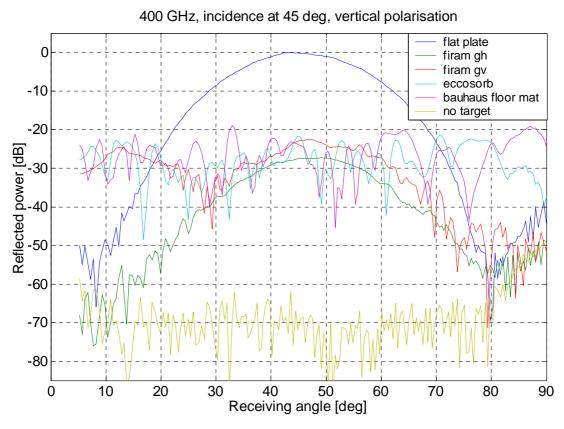
Figure 5.11 Scattered power as a function of the receiving angle (vertical polarisation at 400 GHz,  $\theta_i = 45^{\circ}$ ).
