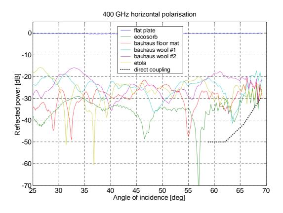
Figure 4.13 Reflectivity as a function of the specular angle at 400 GHz and horizontal polarisation.
