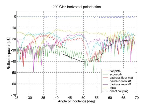
Figure 4.9 Reflectivity as a function of the specular angle at 200 GHz and horizontal polarisation.
