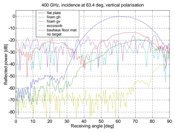
Figure 5.13 Scattered power as a function of the receiving angle (vertical polarisation at 400 GHz,  $\theta_i = 63.4^{\circ}$ ).
