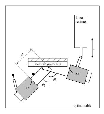
Figure 5.1 Schematic layout of the non-specular reflectivity measurement system.
