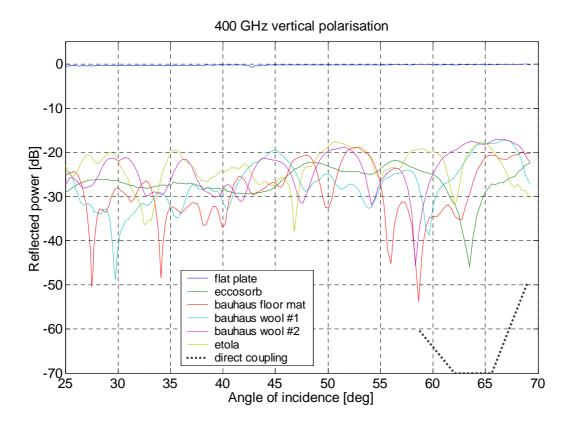
Figure 4.12 Reflectivity as a function of the specular angle at 400 GHz and vertical polarisation.
