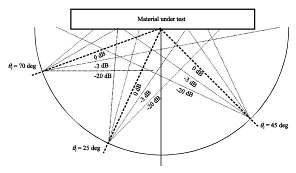
Figure 4.5 Illustration of the sample illumination from the corrugated horns.
