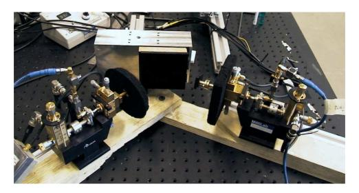
Figure 5.2 Photograph of the non-specular reflectivity measurement system (300 GHz, TK THz RAM,  $\theta_i = 45^{\circ}$  and horizontal polarisation).
