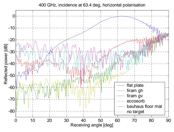
Figure 5.14 Scattered power as a function of the receiving angle (horizontal polarisation at 400 GHz,  $\theta_i = 63.4^{\circ}$ ).
