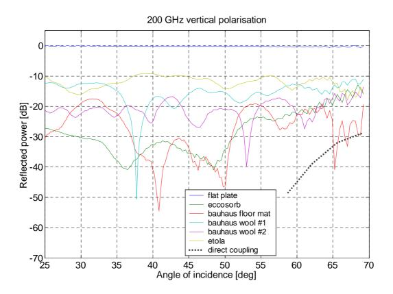
Figure 4.8 Reflectivity as a function of the specular angle at 200 GHz and vertical polarisation.
