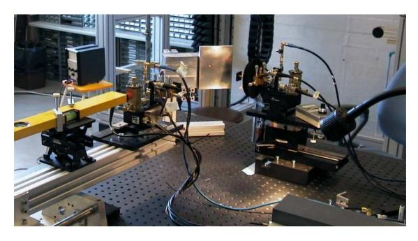
Figure 5.15 Test setup for varying the receivers linear distance from the sample.
