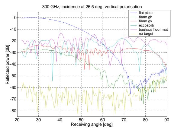
Figure 5.3 Scattered power as a function of the receiving angle (vertical polarisation at 300 GHz,  $\theta_i = 26.5^{\circ}$ ).
