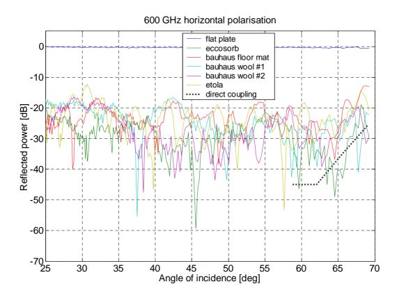
Figure 4.17 Reflectivity as a function of the specular angle at 600 GHz and horizontal polarisation.
