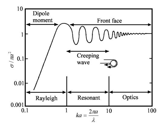
Figure 3.1 Normalized RCS of a metallic sphere (radius = a) as a function of its circumference in wavelengths [2].
