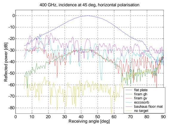
Figure 5.12 Scattered power as a function of the receiving angle (horizontal polarisation at 400 GHz,  $\theta_i = 45^{\circ}$ ).
