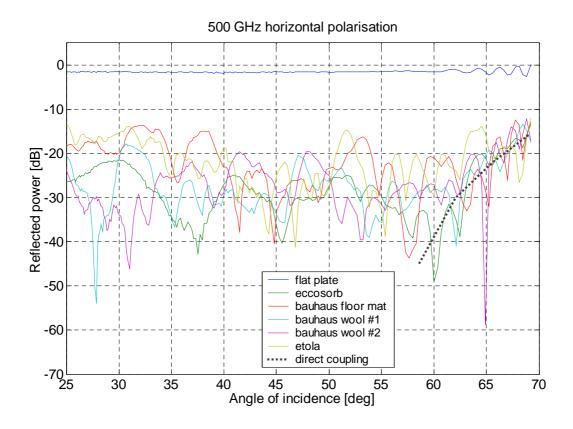
Figure 4.15 Reflectivity as a function of the specular angle at 500 GHz and horizontal polarisation.
