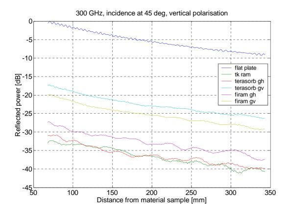
Figure 5.16 Reflected power as a function of the linear distance of the receiver from the sample (300 GHz,  $\theta_i = \theta_o = 45^\circ$ , vertical polarisation).
