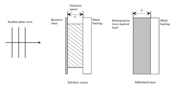
Figure 2.1 Single layer resonant absorbers: the Salisbury screen and the Dällenbach layer.
