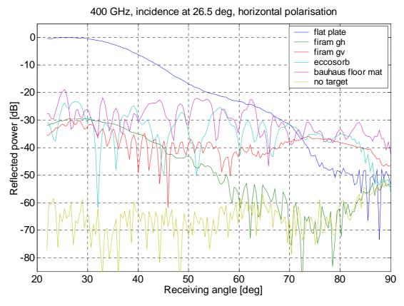
Figure 5.10 Scattered power as a function of the receiving angle (horizontal polarisation at 400 GHz,  $\theta_i = 26.5^{\circ}$ ).
