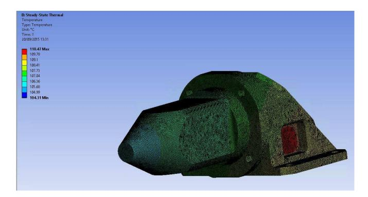
If the heater power is reduced to 5 W a side and the emissivity of the surface increased to 0.8, the temperature increase drops to 30C and – although there are variations across the whole structure, the external cone structure (where the PRT's are) and the inner cone are the same colour in the image below and therefore well within 0.5C
