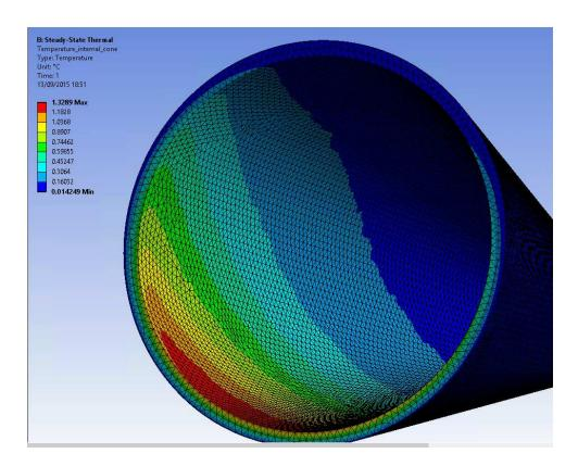
Effect of reflections from the 90 bend structure, with a 100C different environment temperature.
