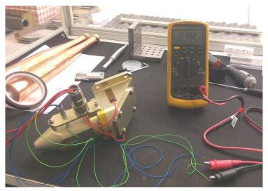
The heater circuits were wired together in parallel and connected to a power supply, which was set to control its output using the voltage it measured. The power supply was set to 26 V output, giving 3.1 W per 218  $\Omega$  heater. (The maximum 28 V for the heaters was just above that achievable by this power supply.)
