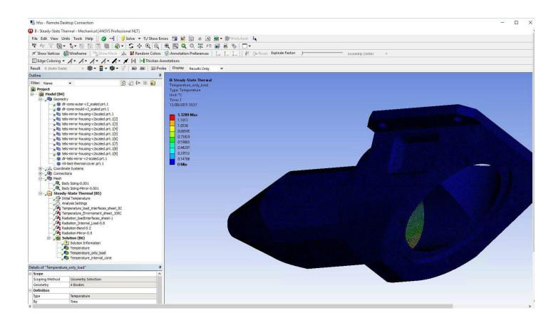
The temperature of the whole body, with the mirror removed to allow one to see inside the structure. And here's the data-tree to set the calculation up.
